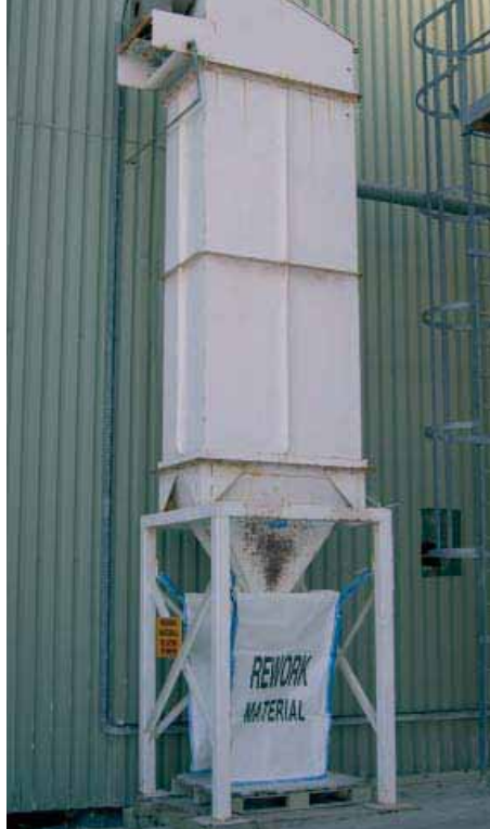
To recycle usable raw material, the contents of SkipVacs and dust collectors goes into “rework” bags to be returned to the relevant stockpile.
